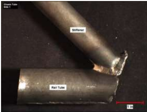
Figure 1: Photograph of failed chassis received for analysis. Side 1 shown.
