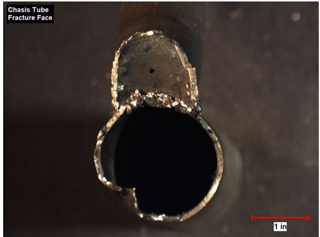
Figure 3: Photograph of failed chassis received for analysis. Fracture face shown in photograph.
