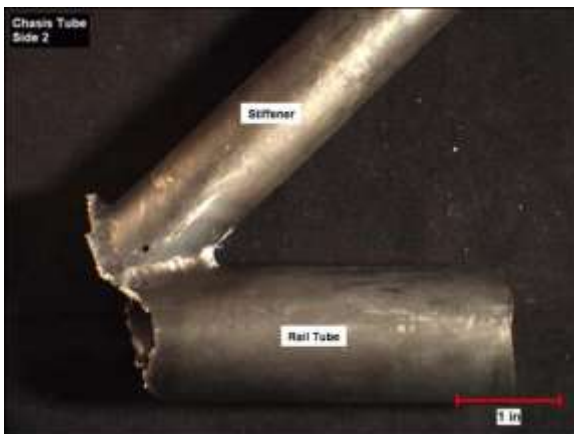
Figure 2: Photograph of failed chassis received for analysis. Side 2 shown.
